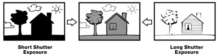
Dual-shutter method combines pixels from short shutter and long shutter images to achieve wide dynamic range.
