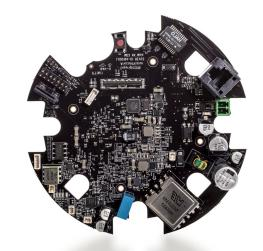
Top: Arecont Vision Costar MegalP integrated circuit board on left, flip side of the IC board on right.
