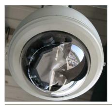
farthest away can be seen in very fine clarity. Axis 209 cameras provide 640x480. Axis 212 models have the 1.3 megapixel image sensor but output VGA so they can have digital Pan and Tilt capabilities. In the Milestone software, Fine can schedule the Pan and Tilt automatically, override it to look in a certain direction, or zoom in digitally to see more details.
