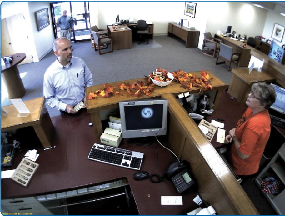
H.264 megapixel cameras eliminate the need for one camera per teller. Security staff can easily identify monetary denominations.
