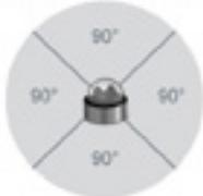
Ultra-compact design incorporates four 2 megapixel sensors for full 180° or 360° coverage.
