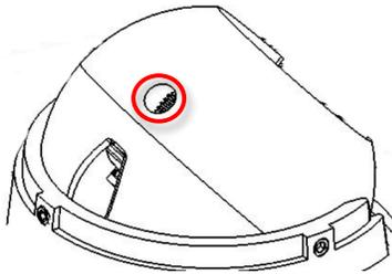
Figure 2: Optional: further tighten three lens lock screws
