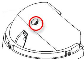
3. Manually unscrew the lens counter clockwise, this may take several seconds.
