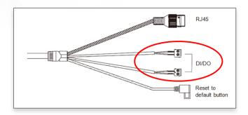
Connect the Alarm In (DI) connector to the alarm input sensor, and connect Alarm Out (DO) connector to the alarm output signal. To avoid any damaged, please follow the specification of the part as below:
