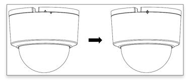
12. Fasten a supplied screw on the dome cover to secure it.
