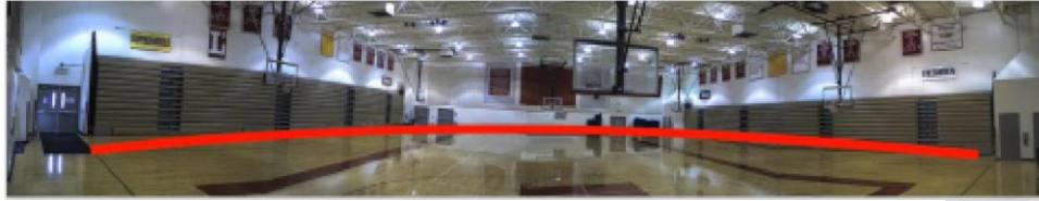
Figure 1D: Mounting height of 8ft and aimed 80ft toward horizon
