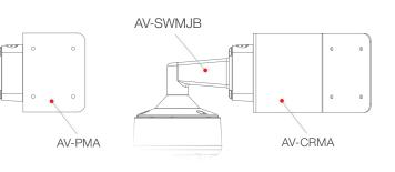
**Wall Mount Configuration** with Corner Mount Adapter
