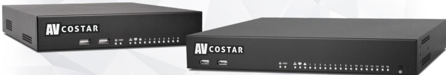
AV Costar™ ConteraCMR® NVR Appliance is designed to offer powerful IP recording in an affordable, compact chassis. The NVR Appliance is equipped with an on-board 8 or 16 channel PoE switch, with a recording capacity of up to 24 channels, allowing for Plug and Play connection with AV Costar and ONVIF cameras or RTSP video streams. With full integration to ConteraWS Web Services, the NVR Appliance offers centralized user management,
