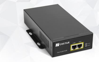
The 7412007-006 is a single port PoE Injector with a wide temperature range and surge suppression for complex high-power requirements. It provides 55VDC, 1.36A power to remote devices over 4 pairs with 6kV (10/700µs) surge protection and supports 10/100/1000Mbps data speed. Compatible with IEEE 802.3af/at/bt compliant 75W PoE devices, such as high-power cameras, wireless access points, base stations, door locks, displays, POS, information kiosks, and other high-power Ethernet terminals.
