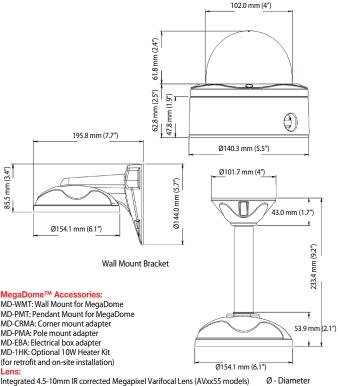
Pendant Mount Bracket Integrated 8-16mm IR corrected Megapixel Varifocal Lens (AVxx55-16 models)
