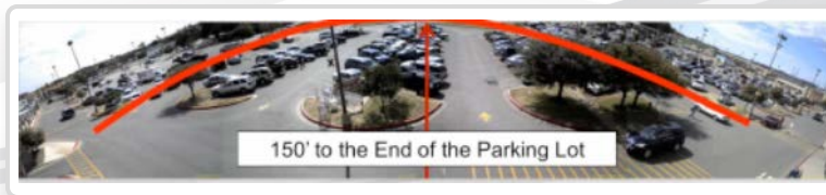
30ft mount and aimed only 150ft toward horizon. Result: Higher curvature produces less desirable results.
