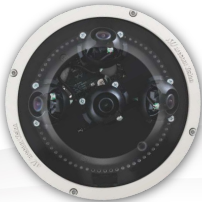
4 Wide Angle Lenses (One pointed to the ground directly below)
