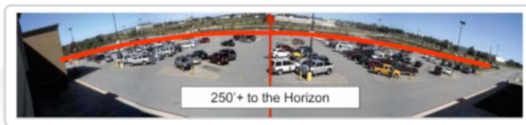
30ft mount and aimed 250ft toward horizon. Result: Less curvature provides better results.
